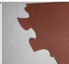
4 Prepreg pre-impregnated fiber. Semi-finished product of carbon or glass fibers and a non-hardened duro- or thermoplastic matrix.
